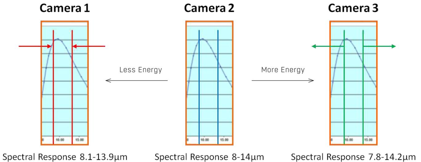
All three cameras "see" slightly different radiant energy levels for the same target temperature. The cameras all read the same as they are calibrated to "understand" that this specific level of intensity equates to a specific temperature, however this will cause an error when used with a spectrally transmitting IR Window.
