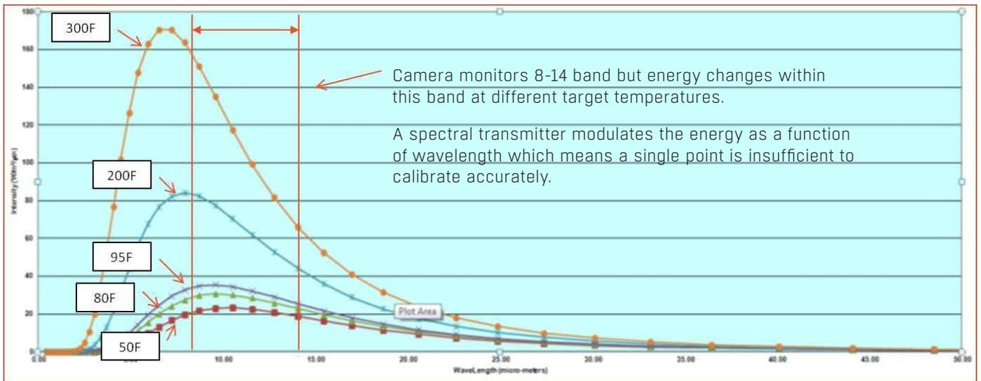
Planck's curve "moves" along the IR Spectrum depending upon target temperature.
